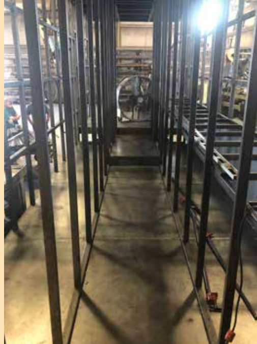
Photo shows instructor access space in center with student space around the perimeter. Two additional levels will be built in the interior.
